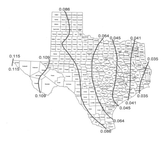
Note: To obtain the application rate for any particular area, refer to the isopleth line to the left of the area.
